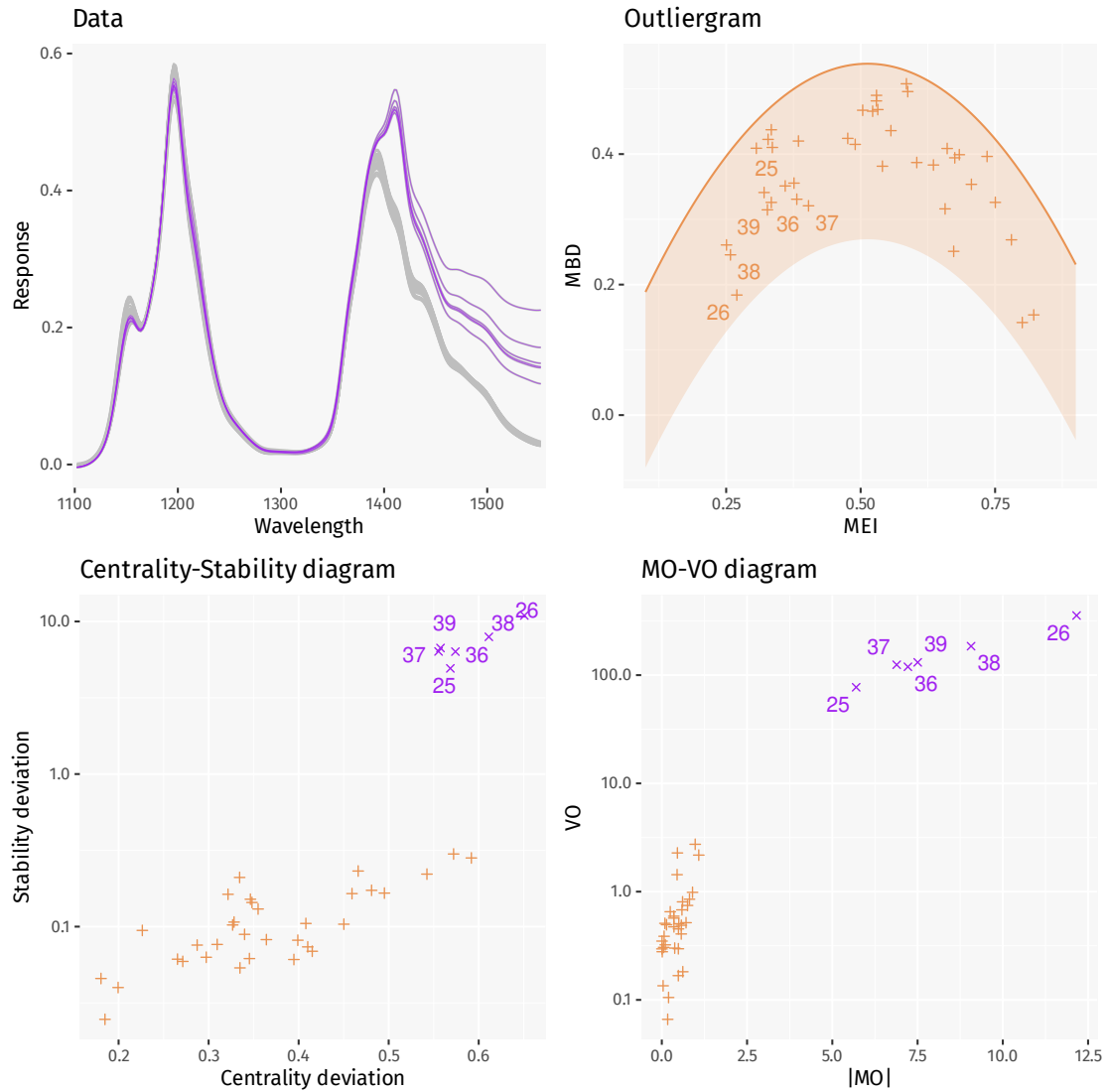
Figure 3.7: Outliergram, centrality-stability, and MO-VO diagrams for the NIR spectra of 39 gasoline samples, from the R package rrcov . The six purple curves #25, 26, 36-39 correspond to samples containing added alcohol. While the outliergram does not clearly identify these outliers, the centrality-stability and MO-VO diagrams show a marked separation from the main curves. Indeed, there is no cutoff d^* defining the lower boundary of the orange ribbon in the outliergram which properly excludes the six outliers.
